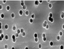
A Fragment of a Track Membrane
