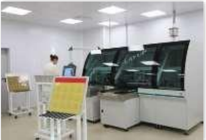
PrintProcess LAYUP 2 assembly- before-pressing system (Switzerland)
