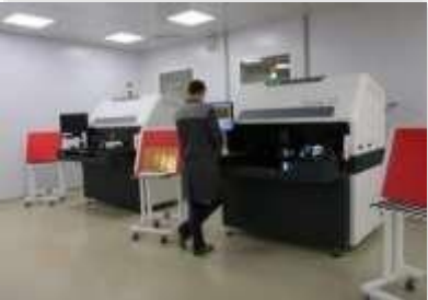
Orbotech FUSION 22 automatic optical control system (Israel)
