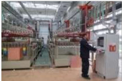
PAL vertical chemical galvanic line (China)
