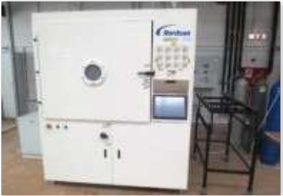
PLASMA MARCH plasma coating machine (United States)
