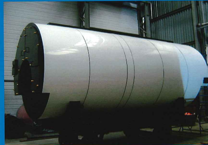
Hot-water boiler “FR10-8-16-204” (8.0 MW, mass – 24 tons) At the territory of production building ready for shipment on railway platform
