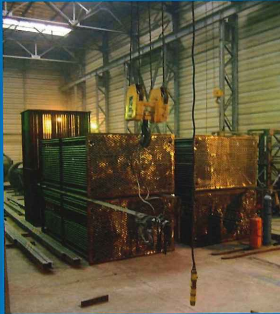
Tubular Air Preheaters for JSC EEK Aksu, Kazakhstan.
