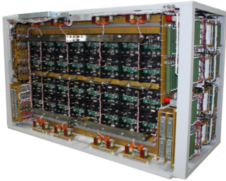
Traction converter 4000kVa
