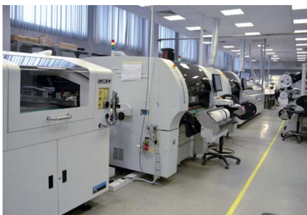
3 Surface Mount lines with 5 Mount Assembly machines Universal (Advantis3 AC-30S, AX-30S, AC-72, AI-07S) with overall productivity of 105 000 components per hour and line of Automated Optical Inspection (AOI)
