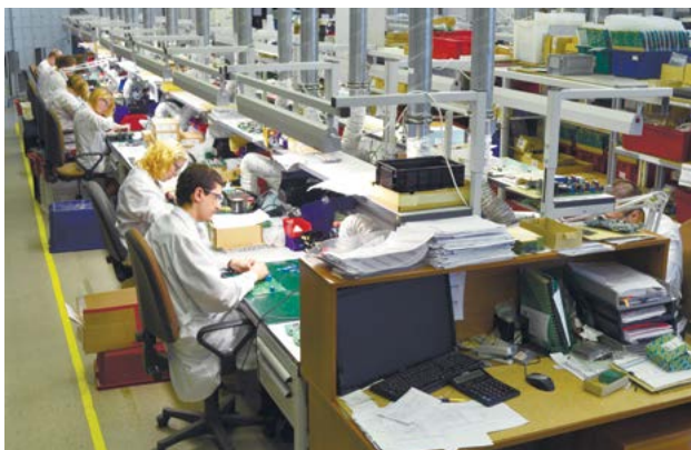
Mounting of terminal components
