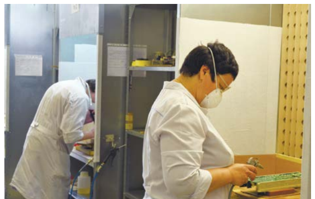
Application of water-proof coating
