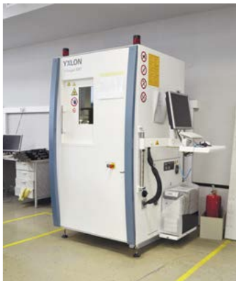
Device for X-ray control Cougar SMT
