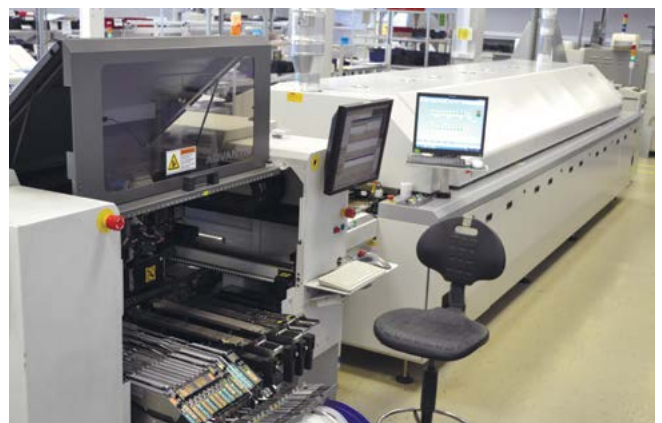
Convection oven of reflow solder JT RS-1000II-N and Vitronics Soltec XPM 2
