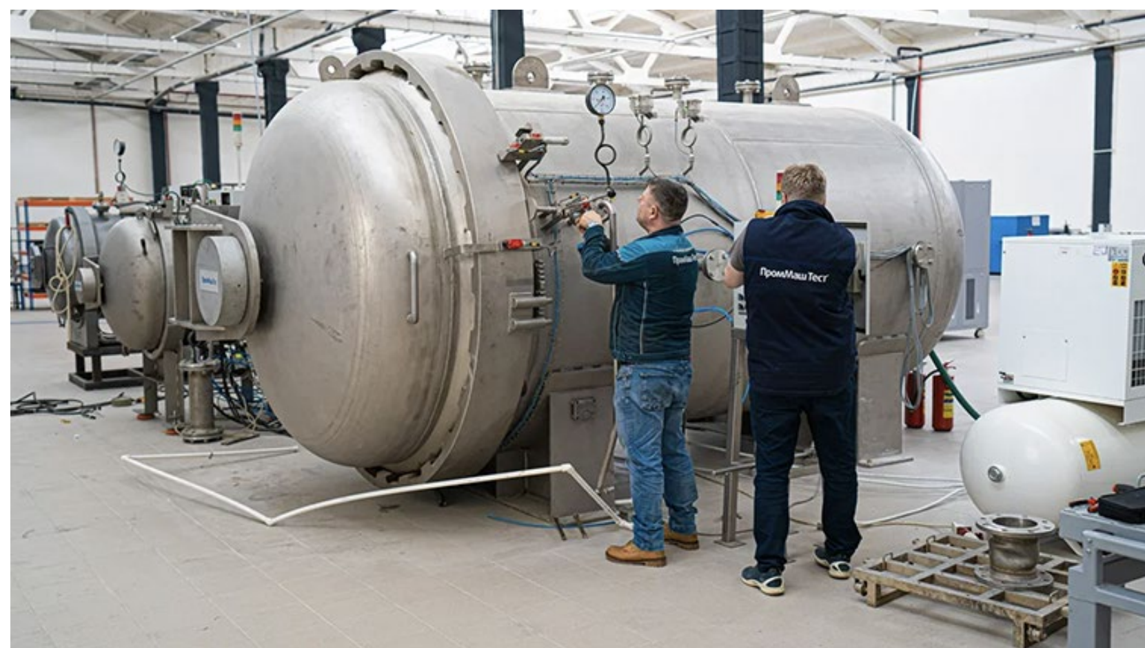
Explosion chambers for investigating the damaging effects of a blast wave
